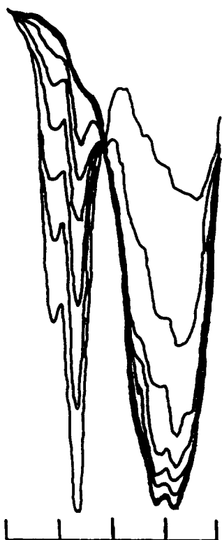
Fig. 1.—Infrared spectra in \text{CHCl}_3 . As the reaction proceeds a band at 1800\text{ cm.}^{-1} (due to the peroxide) is replaced by one at 1700\text{ cm.}^{-1} (due to compound A).
